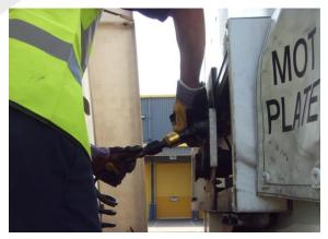
The greatest risk is presented during the coupling of articulated vehicle and trailer combinations. During this operation the driver undertakes activities at the side of the vehicle and/or on the catwalk behind the cab. There is potential for the combination to move, if the tractor unit parking brake has not been applied, when the trailer brake is disengaged or when the red emergency line is connected.
