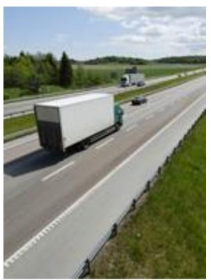
Boxed trailers can be loaded in a variety of ways (see PCSA *Loading Options Guidance Document*) but generally they are loaded from either ground level or a loading dock. They offer substantial load capacity which is well suited to long haul operations and can be loose loaded or loaded with pallets and/or containers allowing the operator to optimise loading.
