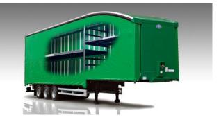
Load planning and distribution is crucial in relation to double deck trailers to maintain an appropriate centre of gravity and ensure that the trailer remains stable while in motion. Lighter loads should always be placed on the upper deck and loads on both decks should always be secured. Drivers will require additional training to ensure they are able to control these vehicles.
