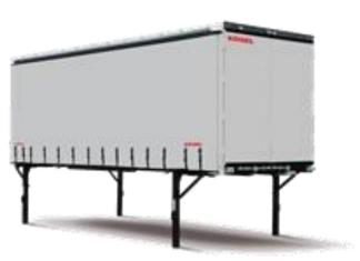
Operators should only consider the use of drop bodies if ground surfaces are firm and level, to ensure they remain stable.
