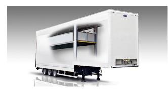
Before selecting double deck trailers operators should consider the routes their vehicles will use as double deck trailers are subject to height restrictions. Operators should also consider the impact of weather conditions on double deck trailers, particularly strong winds.
